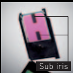
Sub iris The sub iris cuts light leakage.
