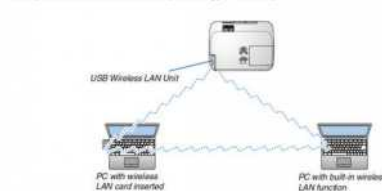
Example of wireless LAN connection (Network Type → Ad Hoc)
