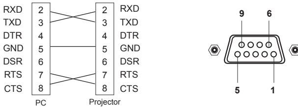
[Figure 1] RS-232 Connection Diagram
