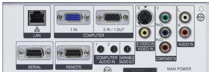
The PT-F100TEA features a LAN connector terminal.
