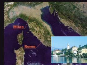
An image of picture-in-picture. A sub picture can be displayed either at the top-left, the top-right, the bottom-left, or the bottom right in the main picture.
