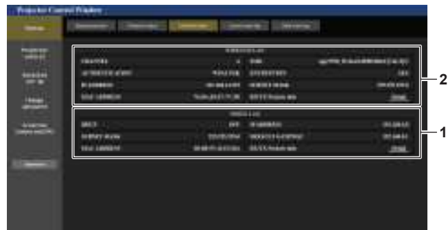
2 [WIRELESS LAN] Displays the settings of wireless LAN when the optional Wireless Module (Model No.: AJ-WM50 Series) is attached.
