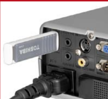
USB terminal which allows users to make PC-free presentations
