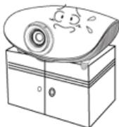
When installing the product in a cabinet or on a shelf, make sure the front end of the base does not protrude.
