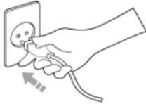
Insert the power plug firmly so that it does not come loose.
