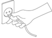
Always unplug the unit by holding the power plug. Pulling the power cable may damage the inside of it.
