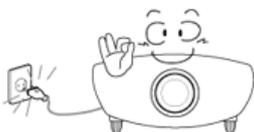
Before moving the product, make sure the power is off and remove the power cord from the wall outlet. In addition, make sure all connection cables are disconnected from other devices before moving it.
