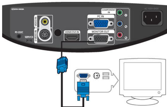
**01** – When using the D-sub (analog) output through another video device (monitor, TV, etc.).
