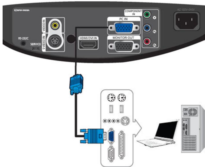
**01** Connect [PC IN] port on the rear side of the projector to the monitor output port of the PC using a PC video cable.
