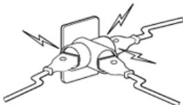
Do not plug multiple devices into a single wall outlet.
