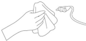
If the power plug pin or jack is exposed to dust, water or alien substances, clean it thoroughly.
