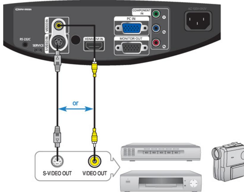
**01** Connect [VIDEO IN(yellow)] input port of the projector to the VIDEO (yellow) OUT port of video equipment using the video cable.
