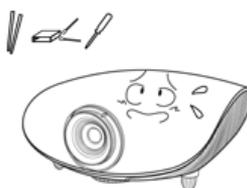
Do not insert metal items, such as chopsticks, steel wire, gimlets, or inflammable objects such as matches or paper into the product through the ventilating openings and the PC/Video and power terminals.
