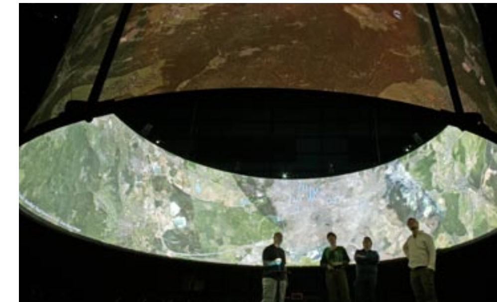
Six projectiondesign F20 sx+ projectors create an 8m wide 360° High Definition display by the ZKM Institute for Visual Media in Karlsruhe, Germany.
