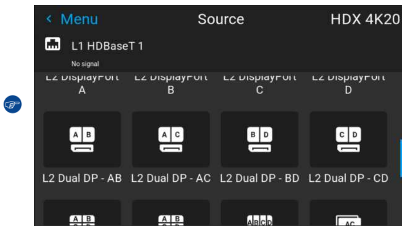
Image 6-5 Example of the stitched input options with the Quad DP board installed
