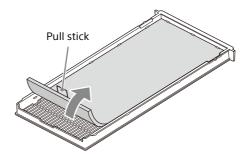
Vacuum the dust from the front side (the side without the pull stick) of the air filter with a vacuum cleaner.
