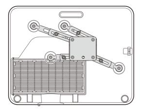
It is recommended to install it so that the ceiling bracket does not overlap on the air filter cover during installation.
